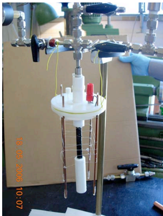
Fig.3. Photo of the Pd-Ag tube after second series of experiments; The cathode, from silver colour, changed to dark one due to salts deposited at its surface.
