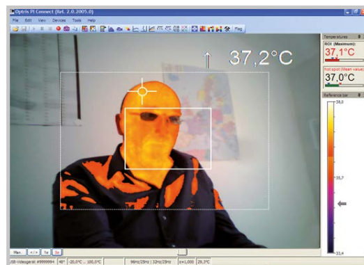
Cross-fading of VIS image above temperatures of 35 °C
